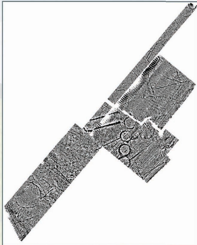
Detailed magnetometry image showing prehistoric features of regional significance (image width approximately 400m; data courtesy of Archaeological Surveys Ltd)
